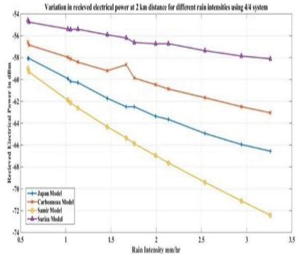
Fig. 8: Variation in received electrical power for multiple channel system
