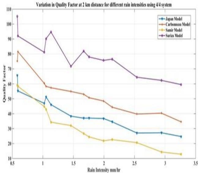
Fig. 10: Variation in Quality Factor for multiple channel system
