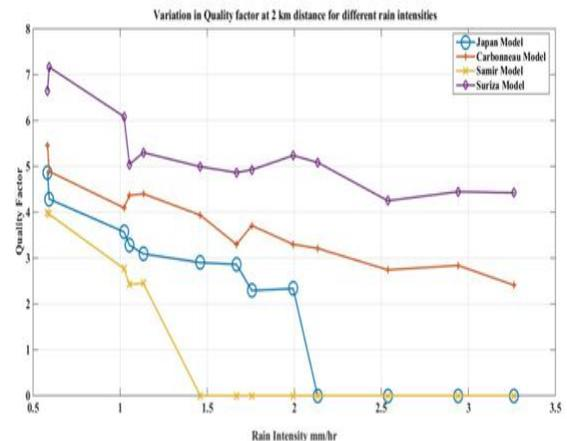
Fig. 9: Variation in Quality Factor for single channel system
