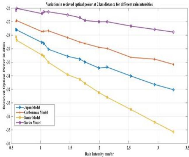
Fig. 5: Variation in received optical power for a single channel system
