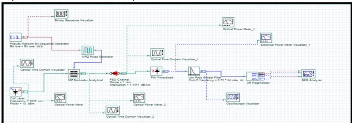
Fig. 1: Single Channel FSO communication system
