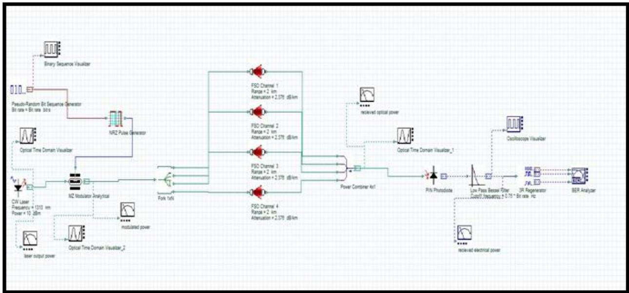
Fig. 2: Four Channel FSO communication system
