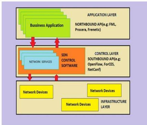
Fig. 1: A three-layer software-defined networking (SDN) architecture
