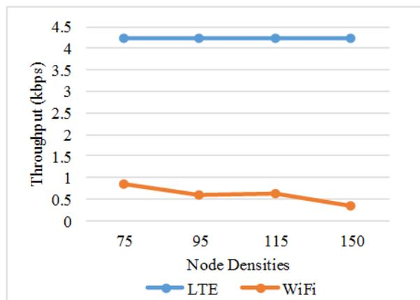
**Fig. 2:** Node Densities vs. Throughput.
