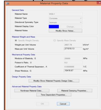
**Fig.3:** Material properties assigning window in ETABS
