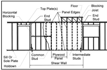
Fig.2: Typical shear wall
