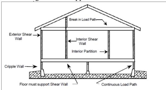
Fig.4: Horizontal alignment of cripple walls
