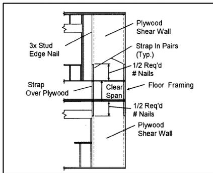
Fig.5: Vertical offset of shear walls
