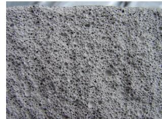
**Fig.1:** Foam concrete
