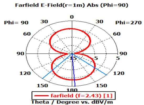
Fig. 13: Angular E-Field at 2.43 GHz.
