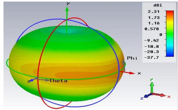
Fig. 12: Directive Gain in ISM Band - 2.43 GHz.
