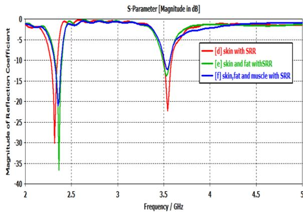
Fig. 8: The Graph Indicated Reflection Coefficient-[D] Skin Layer with SRR [E] Skin and Fat Layer, [F] Skin, Fat and Muscle Layer.
