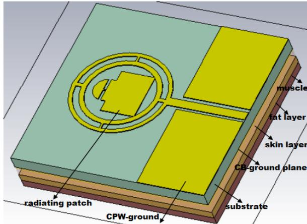
Fig. 3: The Projected Layered View.
