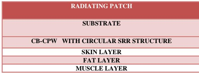
Fig. 2: The Projected Layered Model.
