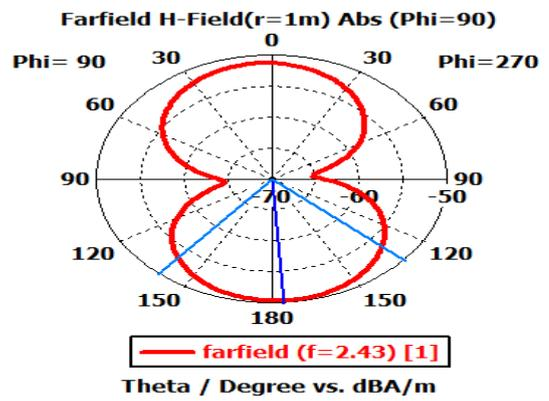
Fig. 14: Angular H-Field at 2.43 GHz.
