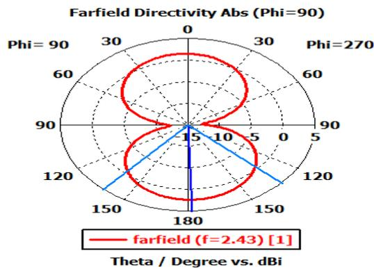
Fig. 15: Angular Plot for Directivity at 2.43 GHz.
