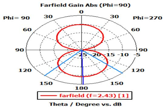
Fig. 16: Angular Plot for Gain at 2.43 GHz.
