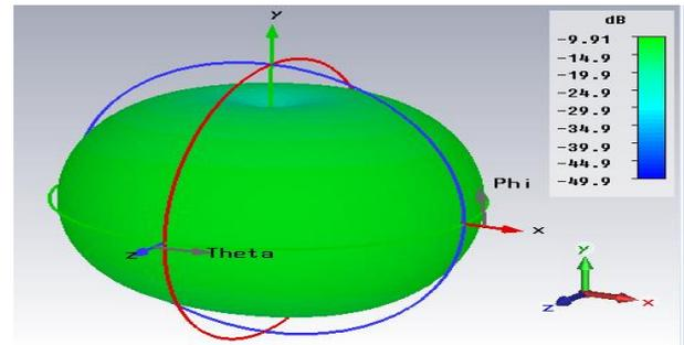
Fig. 11: Gain in ISM Band- 2.43 GHz.
