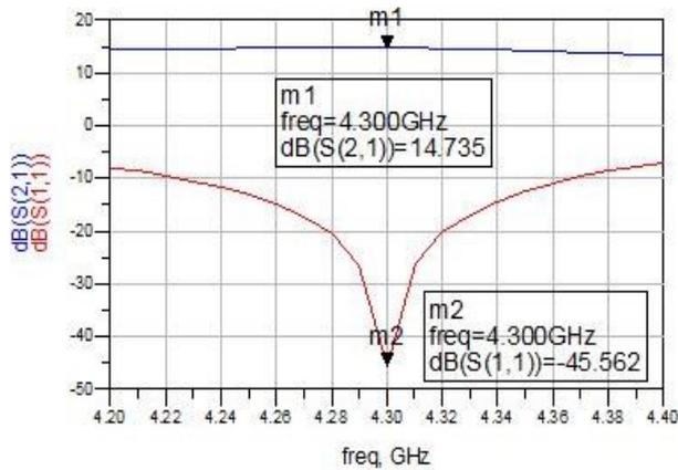
Fig. 7:  $S_{11}$  and  $S_{21}$  of LNA.
