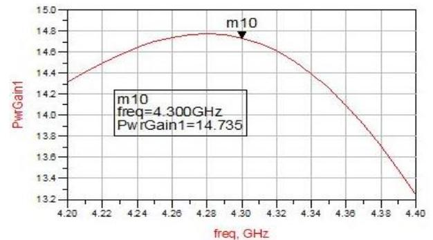
Fig. 4: Power Gain of LNA.
