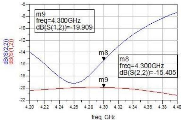
Fig. 8:  $S_{12}$  and  $S_{22}$  of LNA.
