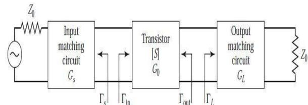
Fig. 1: General Block Diagram of Microwave Amplifier
