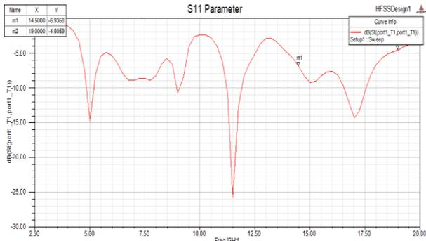
Fig.4: Impedance Bandwidth Plot of Unoptimized 3X3 Array.
