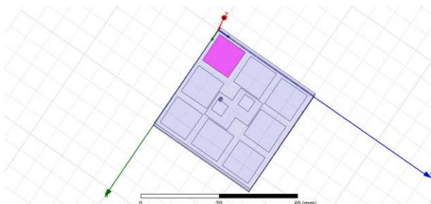
Fig. 1: Geometry of Unoptimized 3X3 Array.
