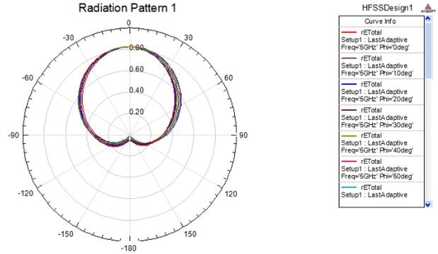
Fig. 8: Radiation Pattern of Optimized 3X3 Array.
