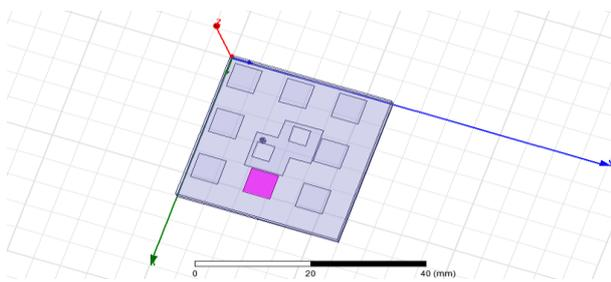
Fig. 2: Geometry of Uptimized 3X3 Array.
