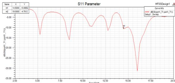
Fig. 7: Impedance Bandwidth Plot of Optimized 3X3 Array.
