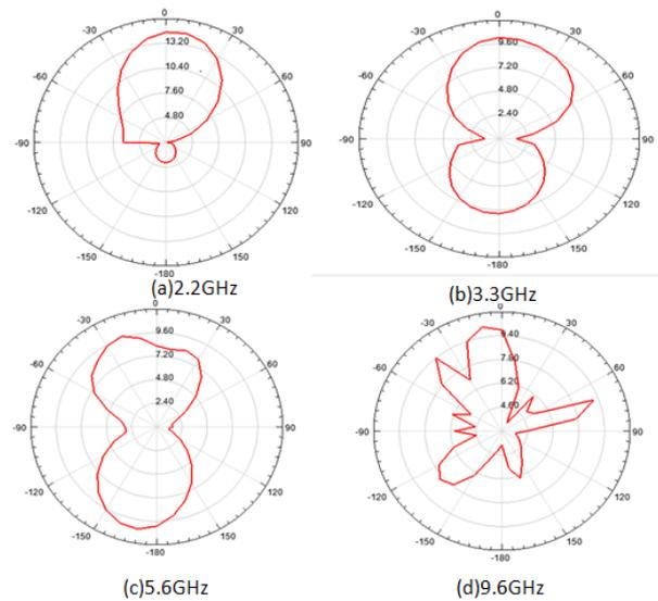
Fig. 6: Radiation Pattern of Antenna at Resonance Frequencies.
