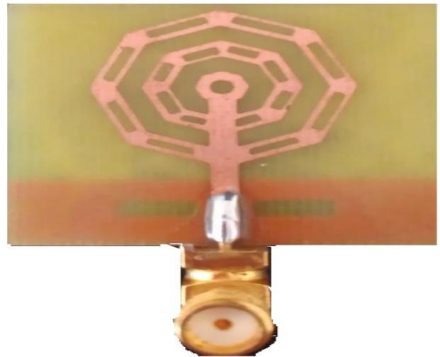
Fig. 3: Fabricated Antenna.
