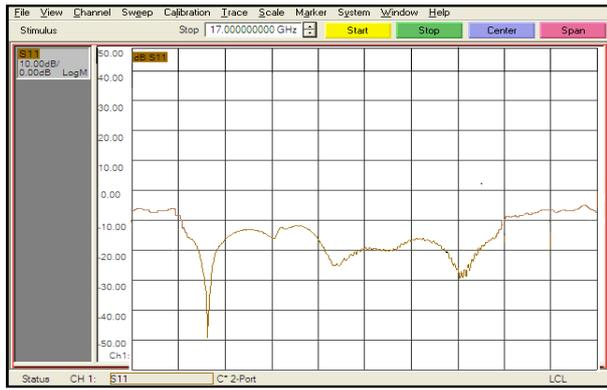
Fig. 4: Measured Reflection Coefficient.
