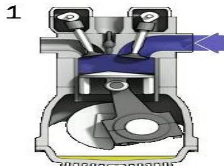
Fig. 1: Intake Operation of Engine.
