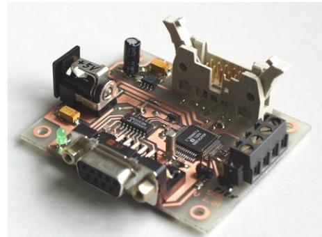
Fig. 5: Developed Circuit of the Sensor and Microcontroller.
