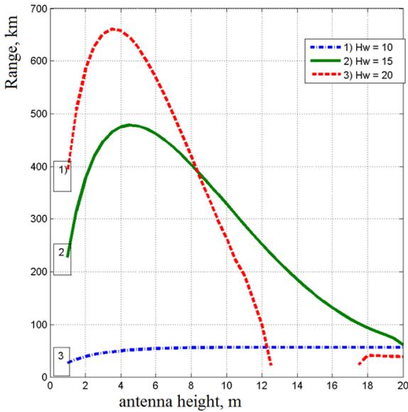
Fig. 4: Range of the radar from antenna height
