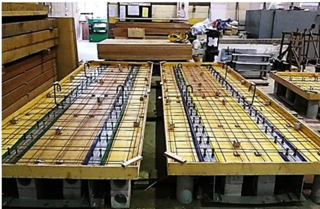
(a) Specimens formwork
