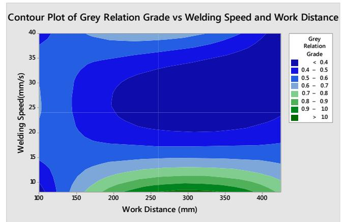
**Figure 6:** Contour plot of grey relation grade Vs welding speed and work distance
