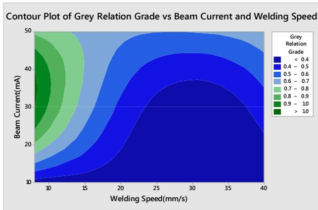
**Figure 4:** Contour plot of grey relation grade Vs beam current and welding speed
