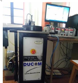
Fig. 5: Pin on disc wear testing machine
