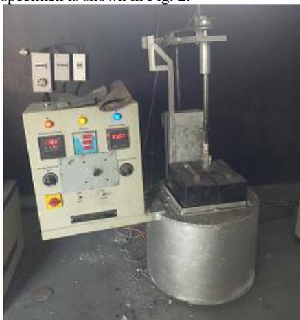
Fig. 2: Stir casting apparatus
