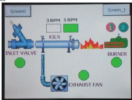
Fig. 5: Front panel HMI screen
