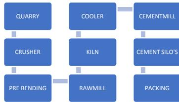
Fig. 1: Process flow chart of cement plant
