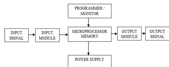
Fig. 3: PLC architecture
