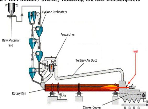
Fig. 2: Block Diagram of kiln with tertiary air duct
