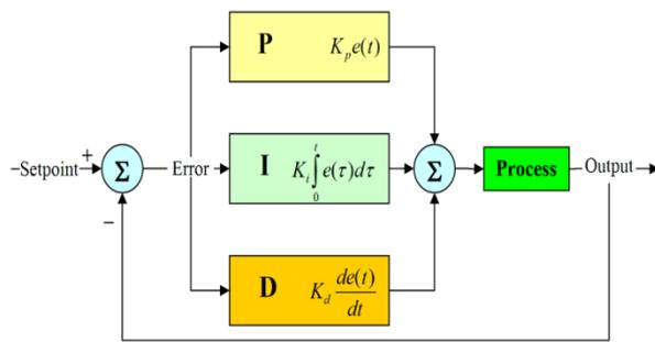
Fig. 4: PID Controller action
