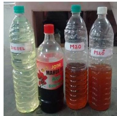
Fig. 1: Diesel and Mahua biodiesel blends
