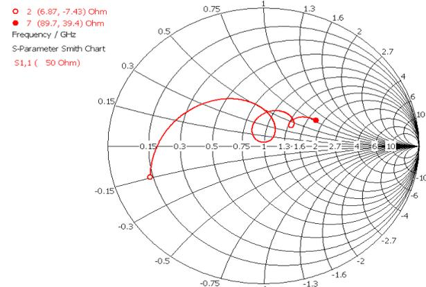
Fig. 4: Smith Chart vs Frequency Plot of Presented Receiver Antenna
