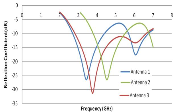
Fig. 3: Reflection Coefficient vs Frequency Plot through Optimization
