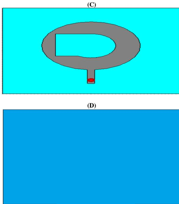
Fig. 1: Proposed Antenna Geometries (A) Antenna 1 (B) Antenna 2 (C) Antenna 3 (D) Ground Plane.
