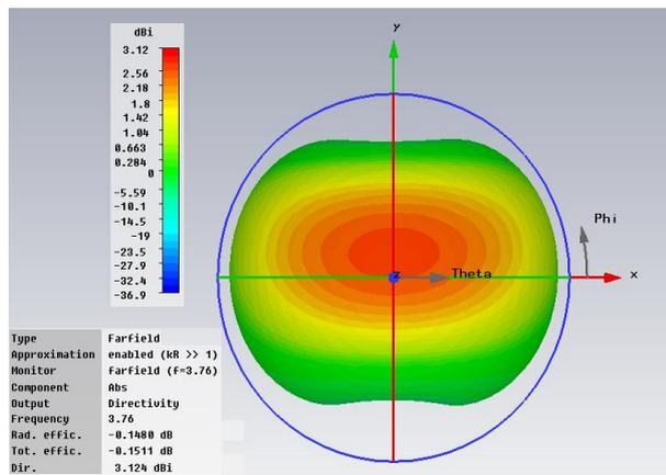
Fig. 6: Far Field 3-Dimensional Radiation Pattern Showing Directivity of Proposed Receiver Antenna.
