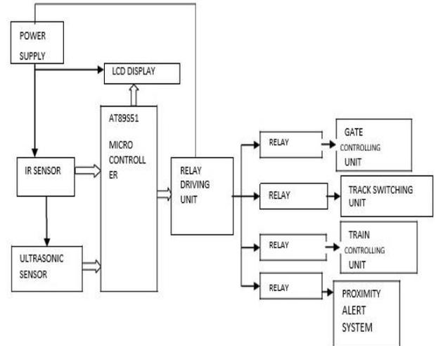
Fig. 3: Diagram of Automated Railway System.
