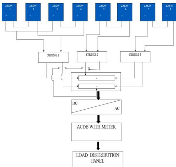
Fig. 2: Layout of Two-20kw Solar Power Plant.
