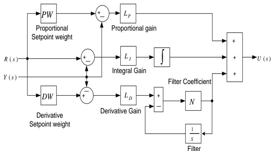
Fig. 2: Organization of Two Degree of Freedom PID (2DOF-PID) Controller.
