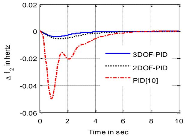
Fig. 7: Oscillations of Area 2 Frequency with Load Enhancement.
