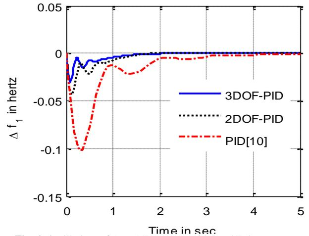
Fig. 6: Oscillations of Area 1 Frequency with Load Enhancement.
