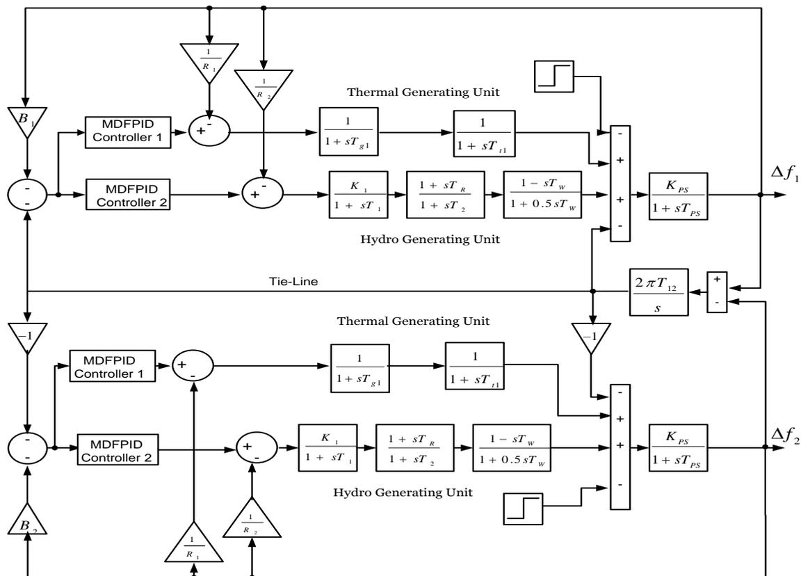
Fig. 1: Two-Area Two-Unit Hydrothermal System Represented by Transfer Function.
