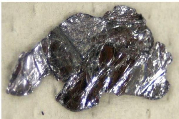
Fig. 1: Molybdenum Di-Sulfide.
