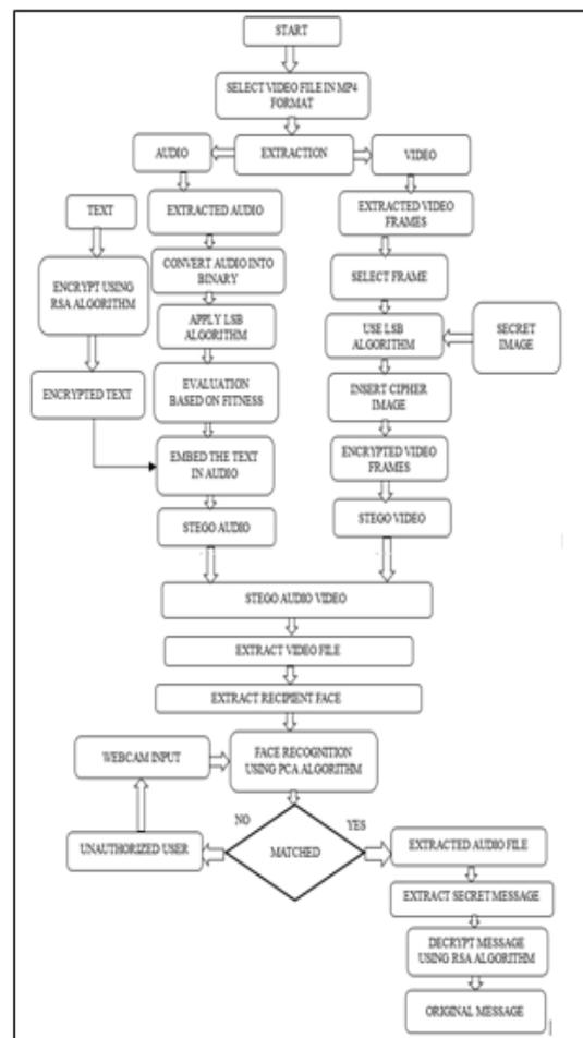
Fig. 3: Flowchart of framework stream
