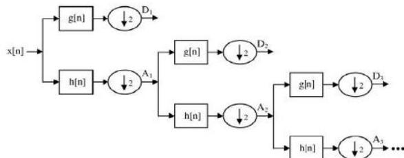
**Fig.1:** Sub-decomposition of Discrete Wavelet Transforms
