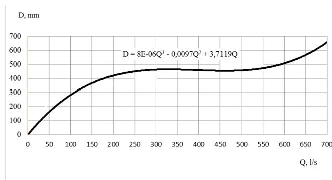
Fig. 4: The chart of dependence between the diameter of polyethylene pipes PE 80 and water expenditure
