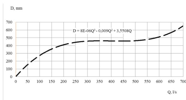
Fig. 5: The chart of dependence between the diameter of polyethylene pipes PE 100 and water expenditure
