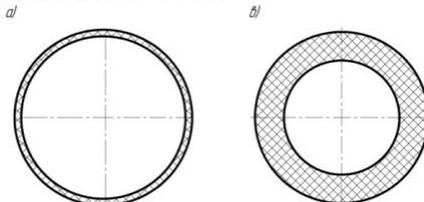
**Fig.1:** The connection between SDR and thickness of a pipe side
