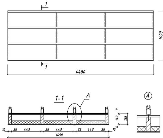
Fig. 3: The two-sided composite skin panel with fastening rails for solar panel.
