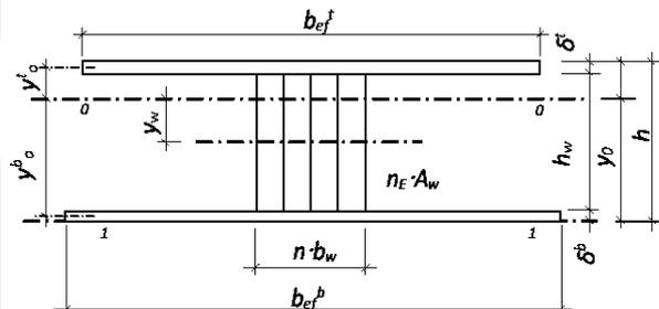
Fig. 5: Transform cross-section as I-beam.
