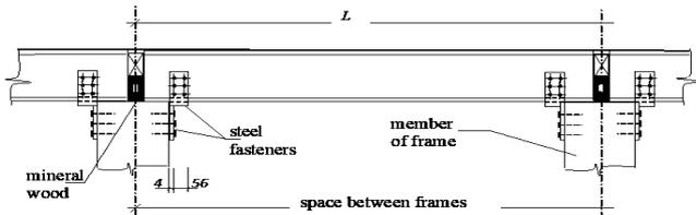
Fig. 4: Fastening composite skin panel to timber members of frame.
