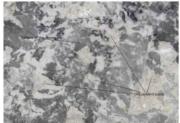
**Fig. 22:** The Microstructure Surface of the Treated CCWA with HCL of 9.0 ML.
