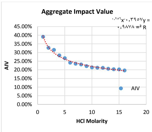
Fig. 28: The Relationship between the HCL Molarity and the Aggregate Impact Value.
