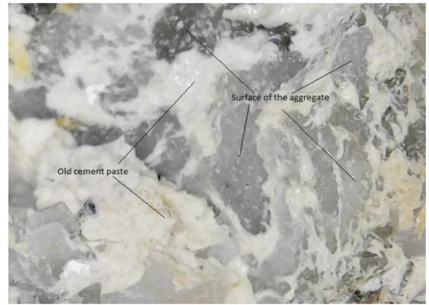
**Fig. 21:** The Microstructure Surface of the Treated CCWA with HCL of 8.0 ML.
