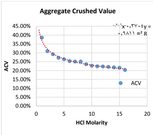
Fig. 27: The Relationship between the HCL Molarity and the Aggregate Crush Value.
