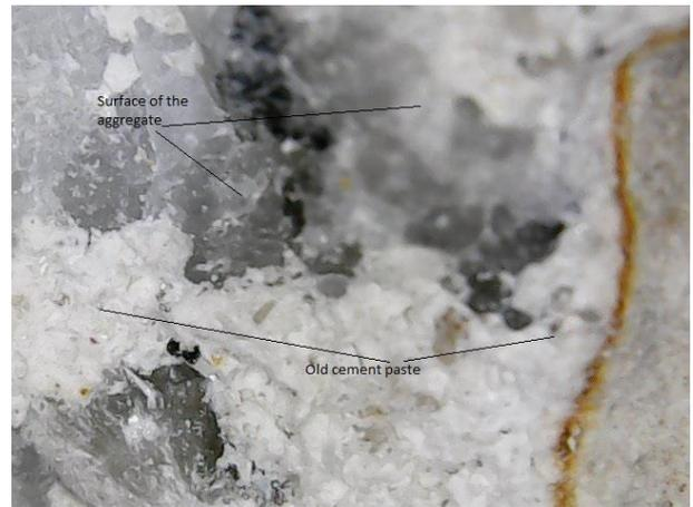
**Fig. 15:** The Microstructure Surface of the Treated CCWA with HCL of 2.0 ML.
