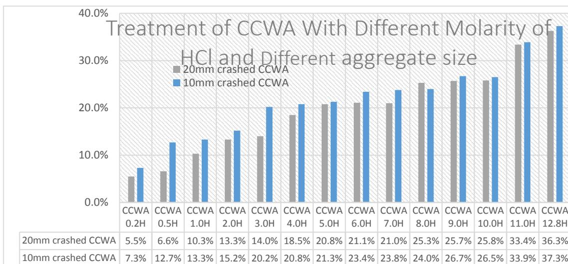
Fig. 6: Treatment of CCWA with Different Molarity of HCL and Different Aggregate Size.
