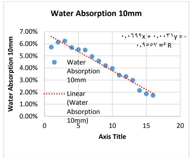
Fig. 30: The Relationship between the HCL Molarity and the Water Absorption 10 MM.
