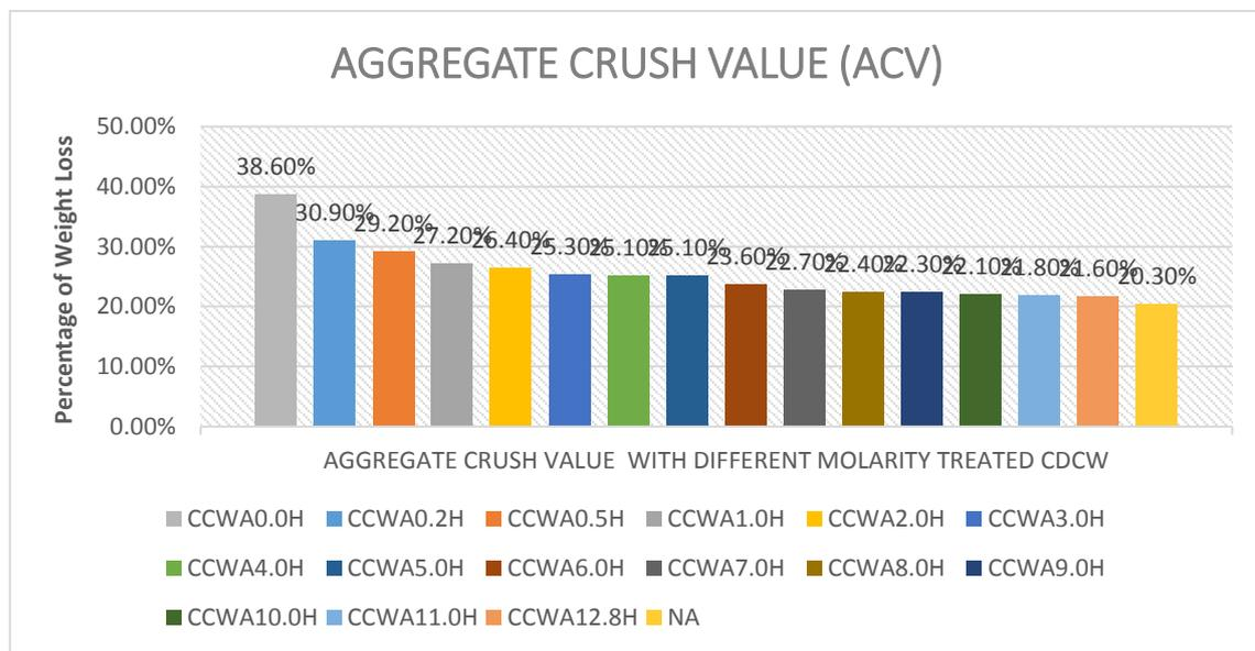
Fig. 7: Aggregate Crush Value with Different Type of Treated CCWA with Different Molarity.
