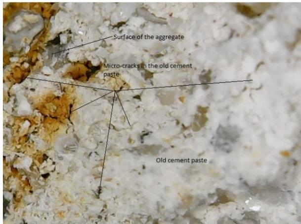
**Fig. 12:** The Microstructure Surface of the Treated CCWA with HCL of 0.02 ML.
