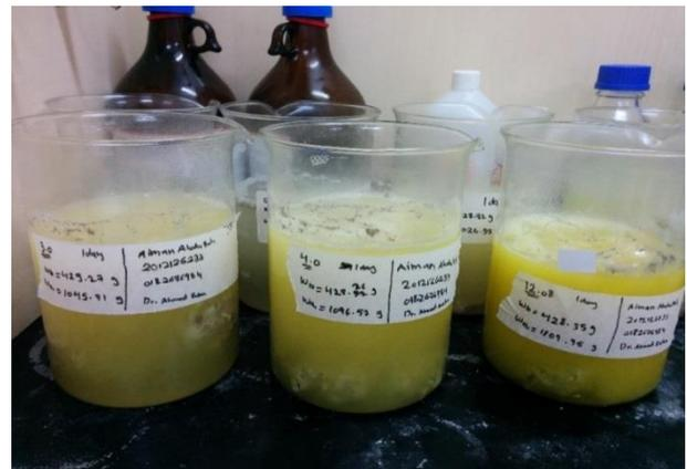
Fig. 3: Specimens of CCWA Soaked the HCL with Different Molarity.
