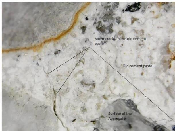
**Fig. 13:** The Microstructure Surface of the Treated CCWA with HCL of 0.05 ML.
