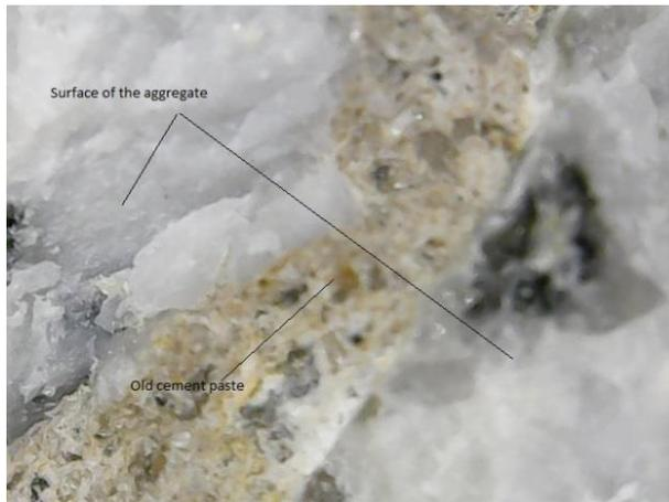
**Fig. 18:** The Microstructure Surface of the Treated CCWA with HCL of 5.0 ML.
