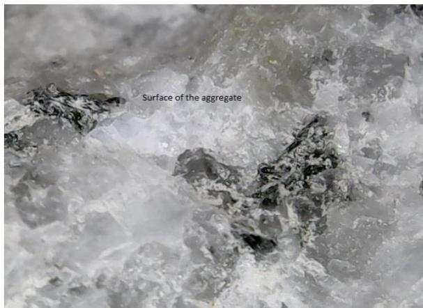
Fig. 25: The Microstructure Surface of the Treated CCWA with HCL of 12.8 Ml.
