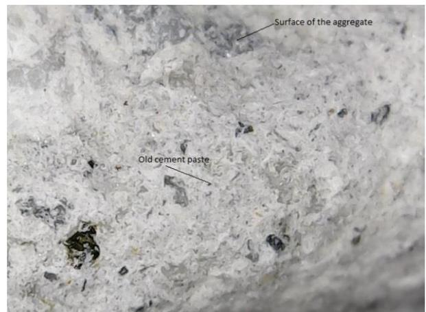
Fig. 11: The Microstructure Surface of the Untreated CCWA.
