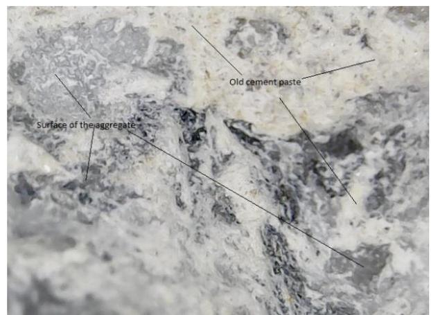
**Fig. 17:** The Microstructure Surface of the Treated CCWA with HCL of 4.0 ML.
