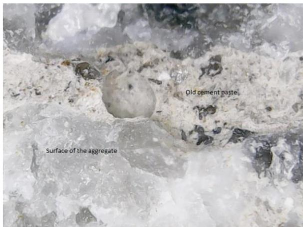
**Fig. 20:** The Microstructure Surface of the Treated CCWA with HCL of 7.0 ML.
