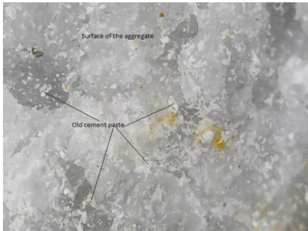
Fig. 24: The Microstructure Surface of the Treated CCWA with HCL of 11.0 Ml.
