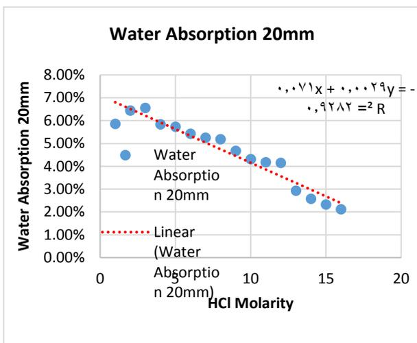
Fig. 29: The Relationship between the HCL Molarity and the Water Absorption 20 MM.
