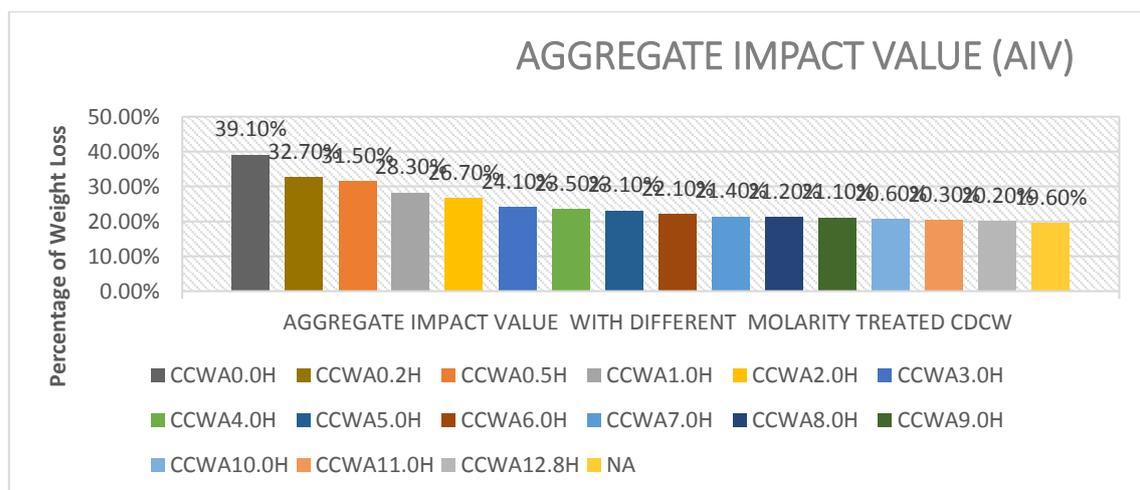
Fig. 8: Aggregate Impact Value with Different Molarity Treated CCWA.
