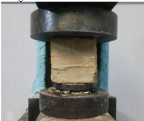
**Fig. 7:** Determination of soil-cement strength
