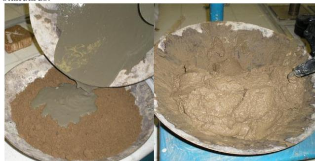
**Fig. 3:** Soil-cement mixture manufacturing
