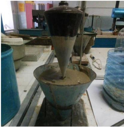
**Fig. 5:** Determination of soil-cement movability by standard cone settle method
