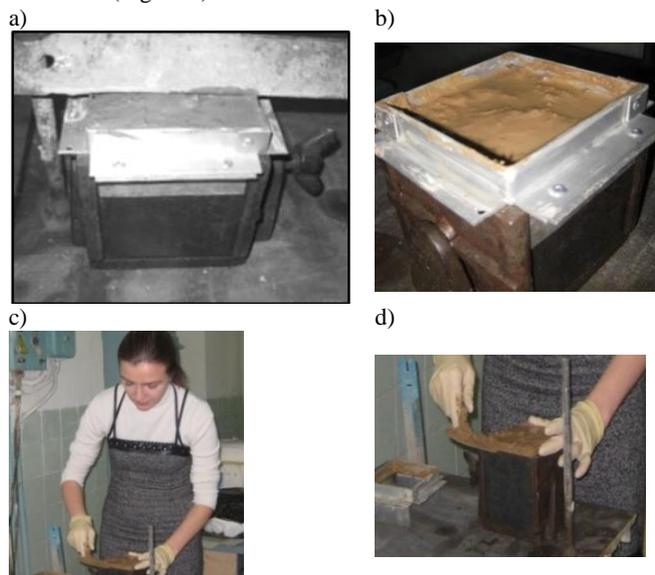
**Fig. 1** Formation of soilcement samples in the form with additional attachment: a) - the beginning of creation, b) - the completion, c, d) - cutting of soil cement remains
