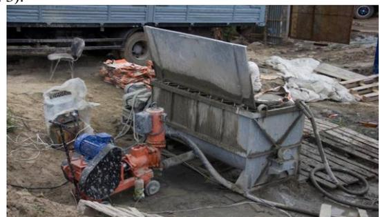
**Fig.3** The complete set of the equipment for supply of water-cement mortar, pump CO-50 and blade mixer.
