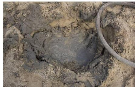
**Fig.7** Condition of the piles of experimental piles one day after placement: a - the pile is made with vibration; b - the pill is made without vibration.
