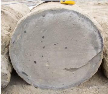
**Fig. 8** Digested experimental cement piles after 28 days after placement: a - the excavated piles; b - a cut of the excavated pile, which was checked.
