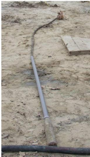
**Fig.5** deep vibrator IV-117 on a flexible shaft.
