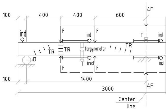
Fig. 1: Scheme of the application of forces and arrangement of measuring devices.
