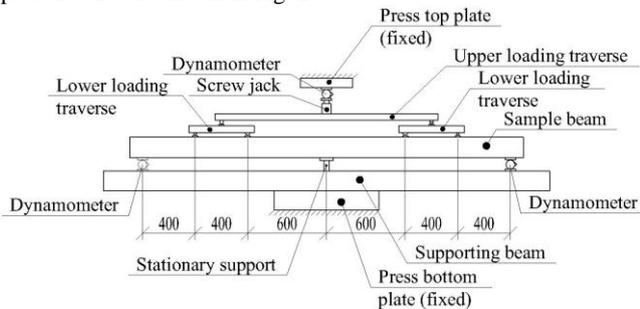
Fig. 2: Test scheme of two-pass beams
