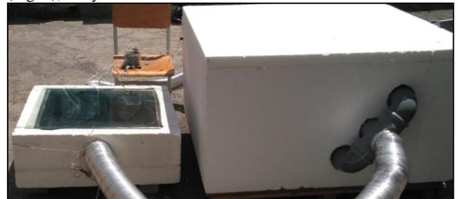
**Fig. 1:** Use of a solar collector for the heat treatment of waterproofing concrete pavement slabs [18]
