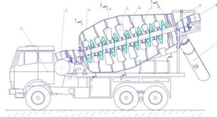
**Fig 1.** The concrete mixer truck of gravity-enforced action with the spiral-blade shaft
