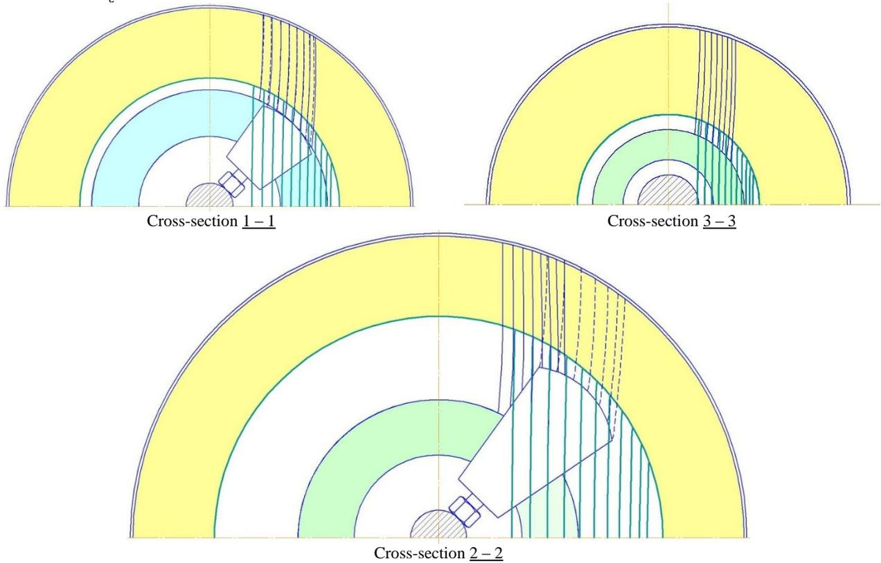
**Fig. 2** The motion path of the concrete mix particles when descending from the screw blades of the drum and spiral-blade shaft of the concrete mixer truck not tacking into account the environmental resistance in three different section of the drum
