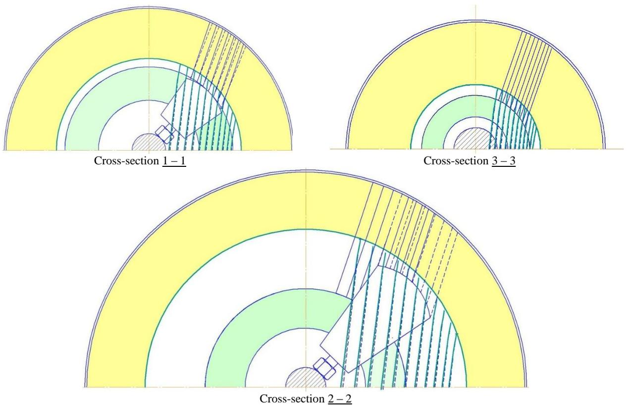
**Fig. 3** The motion path of the concrete mix particles when descending from the screw blades of the drum and spiral-blade shaft of the concrete mixer truck not tacking into account the environmental resistance in three different section
