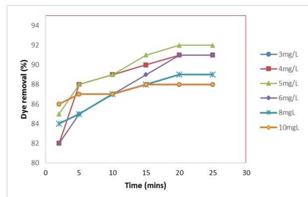
Fig. 3: Time/Concentration Effect of Methylene Blue Adsorption onto Date Palm Leaf Powder at Room Temperature ( $25 \pm 0.5$  °C), Dosage 0.20 G, Ph = 6.0 and Stirring Speed = 1300 Rpm.
