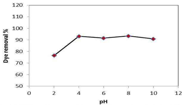
**Fig. 4:** PH Effect of Methylene Blue Adsorption onto Date Palm Leaf Fibers at Room Temperature ( $25 \pm 0.5$  °C), Adsorption Dosage = 200 Mg, Time = 20 Min, Initial Dye Concentration = 4 Mg/L And Stirring Speed = 1300 Rpm.
