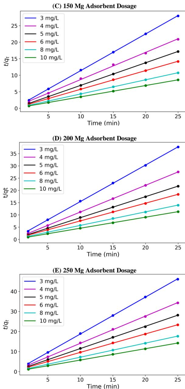
**Fig. 6:** Pseudo-Second Order Kinetics Plot for the Adsorption of Methylene Blue onto Date Palm Leaf Fibers at Different Adsorbent Dosage.
