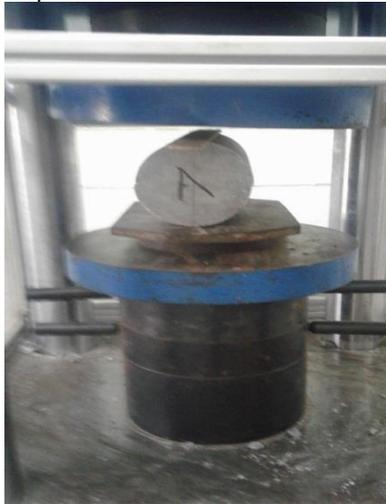
Fig. 2: Splitting tensile test set-up
