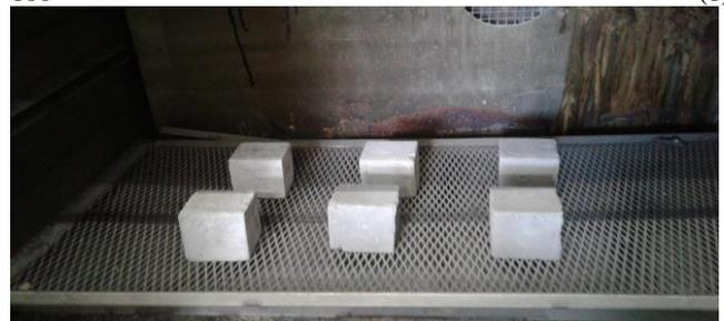
Fig. 1: Oven drying samples for water absorption test
