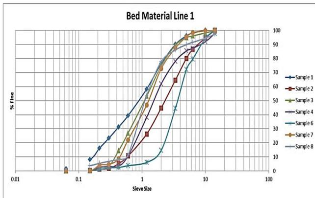
Fig. 2: S-curve of bed material obtained from Sungai Perak.
