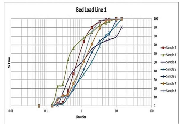
Fig. 1: S-curve of bed load obtained from Sungai Perak.
