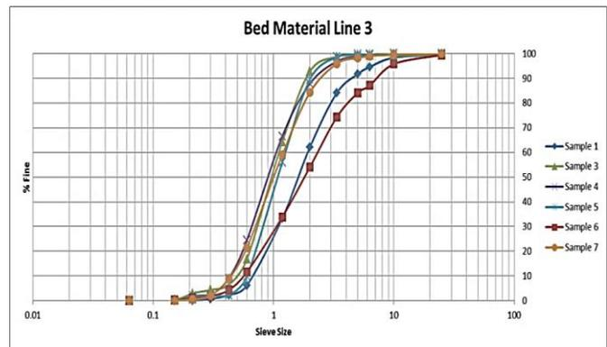
Fig. 4: S-curve of bed material obtained from Sungai Kurau.
