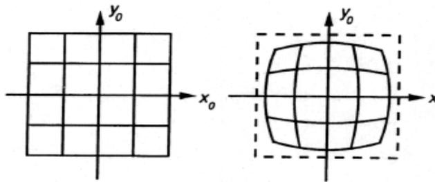
Without Distortion Barrel Distortion
