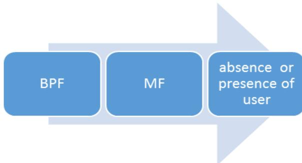
**Fig. 2:** Matched Filter Technique for Spectrum Sensing.
