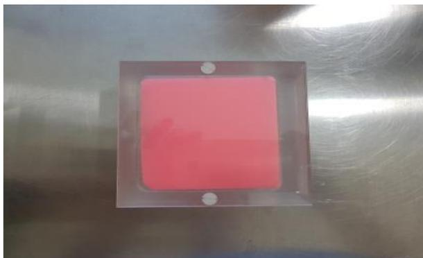
Fig. 3: Breast Equivalent Material Phantom.
