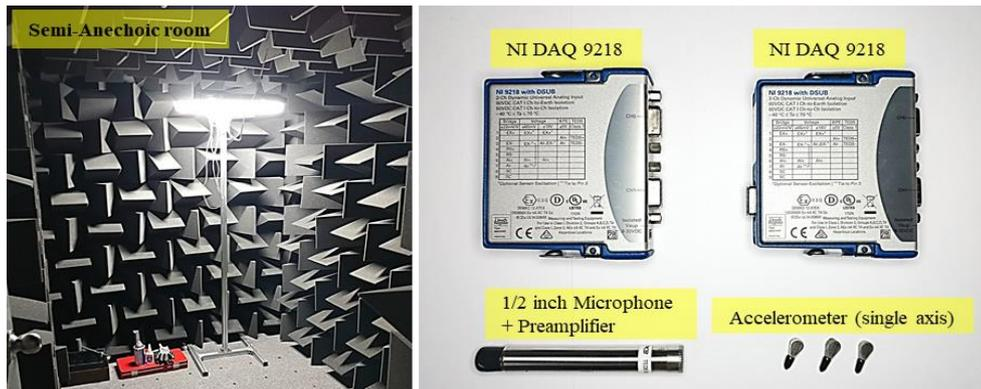
Fig 2: Test Room, Measurement Equipment and Sensors.
