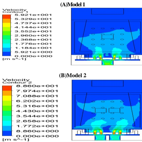
Fig. 7.:Speeds In Air Paths of Models (Input Speed Of 30m/S).
