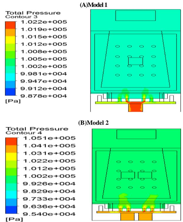
Fig. 9.:Pressure Levels in Air Paths of Models (Input Speed of 30m/S).
