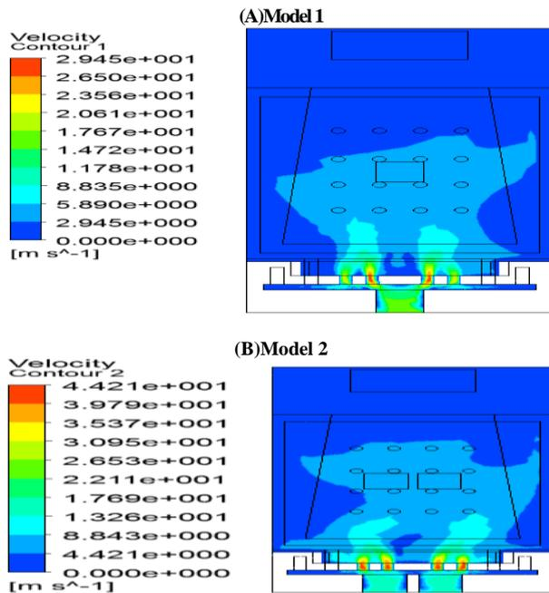
Fig. 6.:Speeds in Air Paths of Models (Input Speed Of 15m/S).
