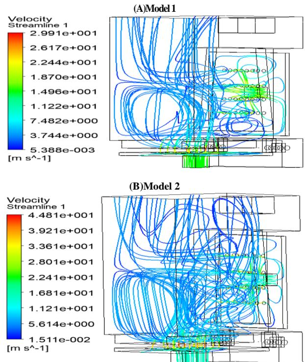
Fig. 4: Speeds in the Entire Shapes of Models (Input Speed of 15m/s).
