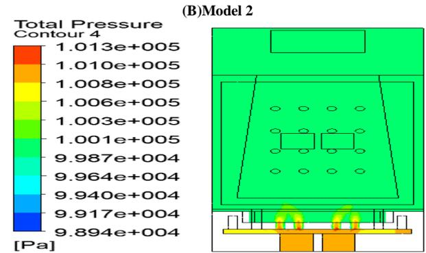
Fig.: 8.Pressure Levels in Air Paths of Models (Input Speed of 15m/S).
