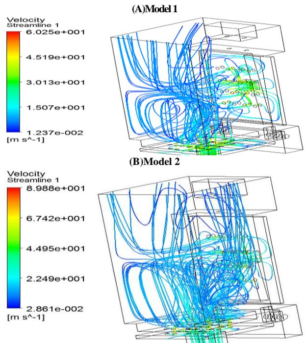
Fig. 5: Speeds in the Entire Shapes of Models (Input Speed of 30m/s).
