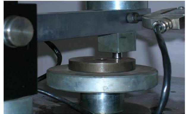
Fig. 22: Pin on Disc Type Wear Testing Machine.
