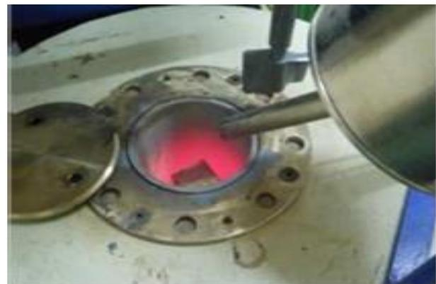
Fig. 8: Al 6061 and NCG Liquid Formation in the Furnace.
