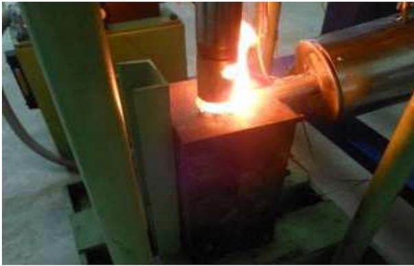
**Fig. 9:** Squeeze Displaced to Casting.
