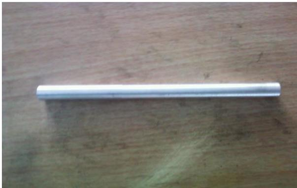
**Fig. 11:** Specimen Obtained by the Lathe Machining Process in Turning Operation.
