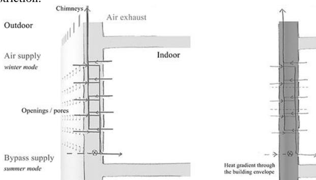
**Fig. 3:** Bio-inspired envelop design for heat retention in cold climate, reproduced from Badarnah (2012).
