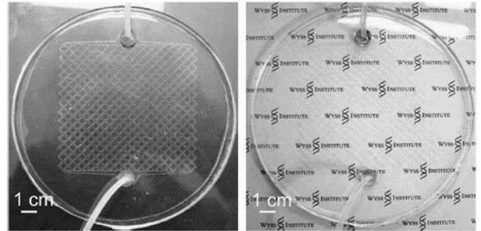
**Fig. 2:** The transparent fluid-filled microtubes run through the window without affecting the clarity of visibility, reproduced from Hatton et al. (2013).
