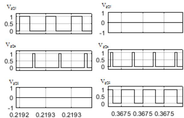
Fig. 6: Gate Pulses for Switches during (a) Boost Mode, (b) Buck Mode.
