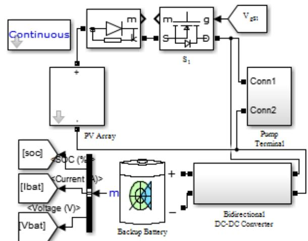
Fig. 3: Simulation Diagram of the Proposed Water Pumping System.
