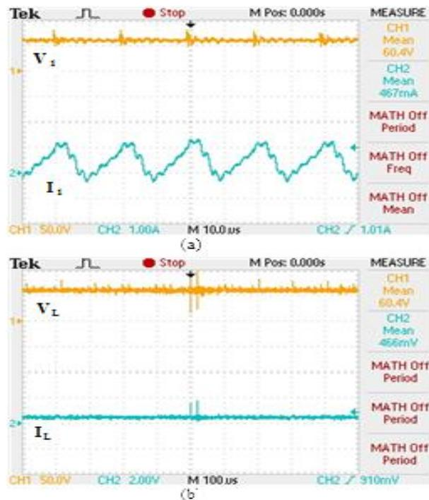
**Fig. 13:** Waveforms of (a) Voltage and Current at Battery Terminal (b) Voltage & Current at Water Pump Terminal in Buck Mode.
