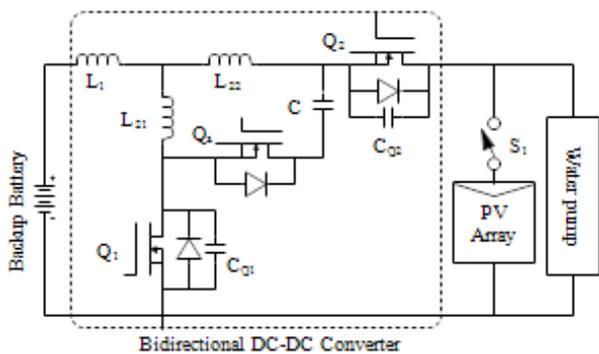
Fig. 2: Schematic Diagram of the Proposed Water Pumping System.
