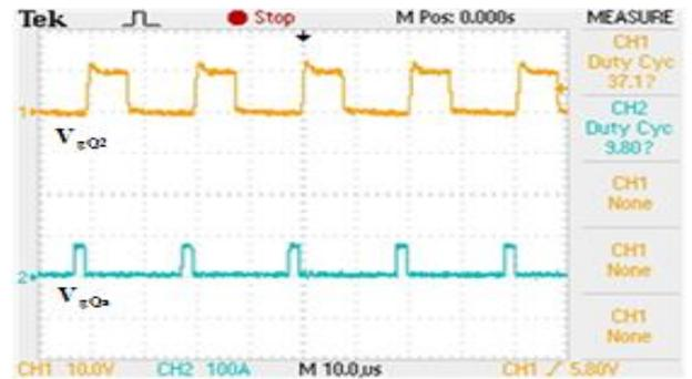
**Fig. 11:** Waveforms of Gate Pulses for Switches  $Q_2$  &  $Q_a$  in Buck Mode.
