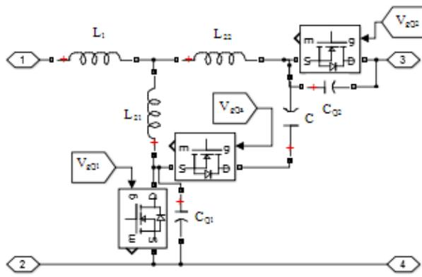
Fig. 4: Simulation Diagram of Bidirectional DC-DC Converter.
