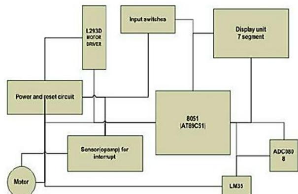
Fig. 2: Block Diagram of the Temperature-Controlled DC Fan [2].
