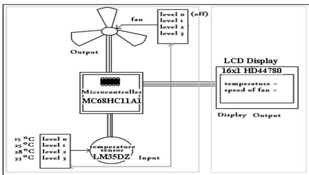
Fig. 1: Block Diagram of Automatic Fan System [1].
