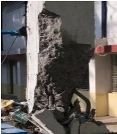
Fig. 8: Crushing of Conventional Column.
