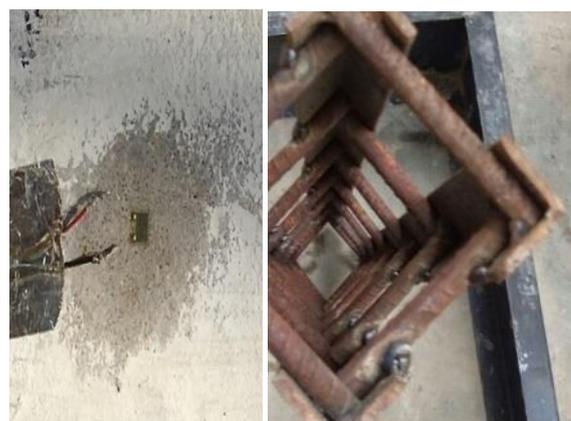
**Fig. 2:** Strain Gauges Attached to Concrete Surface and Reinforcement Showing Welding Connection.
