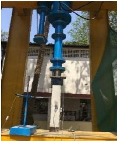
Fig. 3: Testing Setup of Column Specimen.
