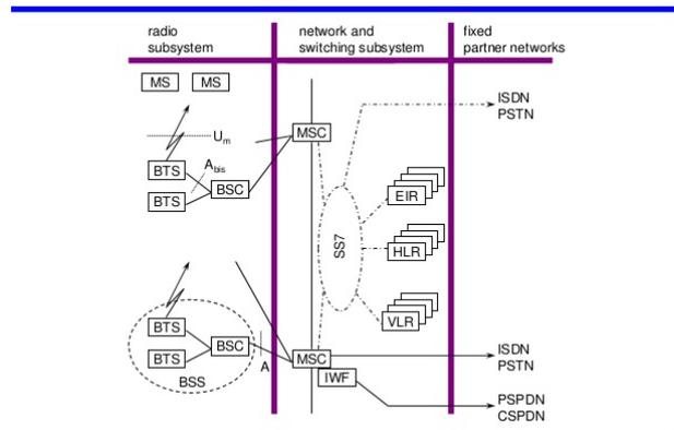
Fig 2. GSM System architecture
