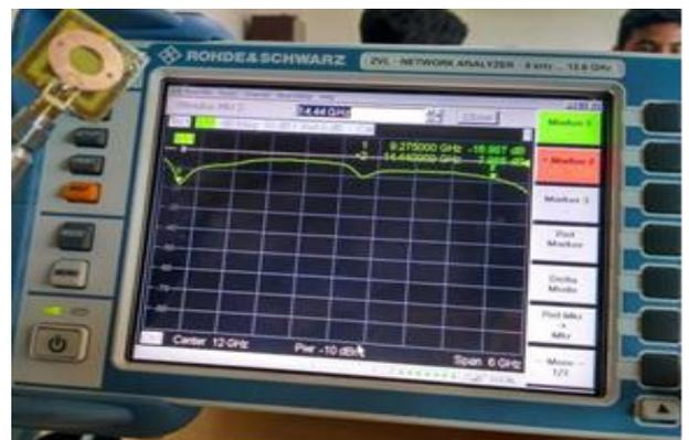
Fig. 6: Photograph of Experimental Set Up to Test Metamaterial Loaded FR4 Based Circular Ring Micro strip Antenna.
