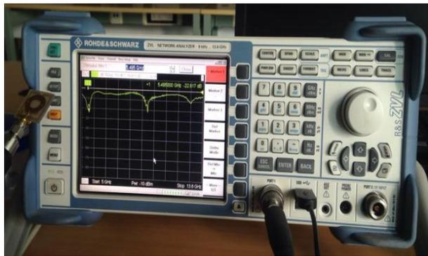
**Fig. 9:** Photograph of Experimental Set Up to Test Metamaterial Loaded RT Duroid Based Circular Ring Microstrip Antenna
