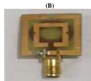
Fig. 4: Photographs of Fabricated Metamaterial Loaded Circular Ring Micro Strip Patch Antenna on RT Duroid Substrate A) Radiating Patch B) Ground Plane.
