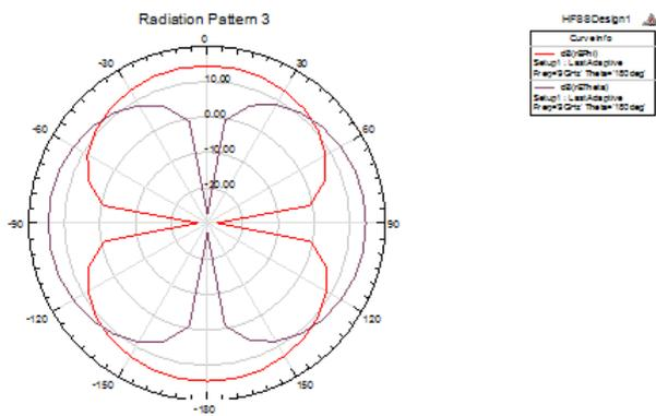
**Fig. 8:** Simulated A) Return Loss B) VSWR C) Gain D) Directivity E) Radiation Pattern At 0o F) Radiation Pattern at 90o G) Radiation Pattern at 180oon RT Duroid Substrate.
