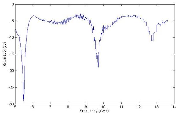
**Fig. 10:** Measured Return Loss ( $S_{11}$ ) Characteristics on RT Duroid Substrate.
