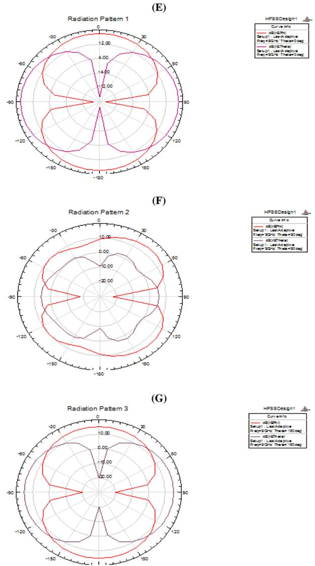
Fig. 5: Simulated A) Return Loss B) VSWR C) Gain D) Directivity E) Radiation Pattern at 0o F) Radiation Pattern at 90o G) Radiation Pattern at 180o on FR4 Substrate.
