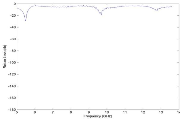
Fig. 7: Measured Return Loss (S11) Characteristics on FR4 Substrate.
