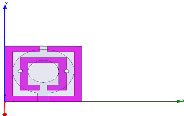
Fig. 1: Geometrical Structure of Metamaterial Loaded Circular Ring Antenna.
