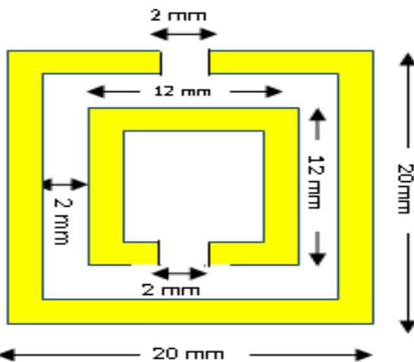
Fig. 2: Geometrical Structure of CSRR Etched on the Ground Plane.
