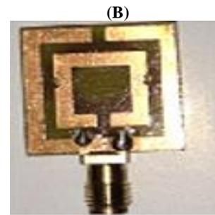
Fig. 3: Photographs of Fabricated Metamaterial Loaded Circular Ring Microstrip Patch Antenna on FR4 Substrate A) Radiating Patch B) Ground Plane.
