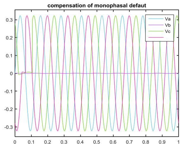
**Fig.6** Simulation of a Monophasal Fault on Grid.
