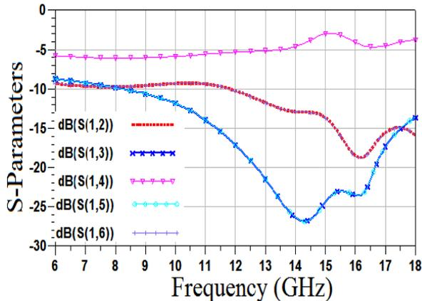
Fig. 9: Insertion Loss of the Proposed Design.
