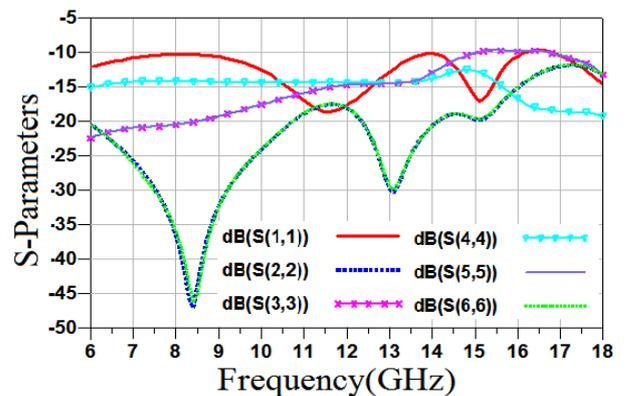
Fig. 7: Return Loss of the Proposed Design.
