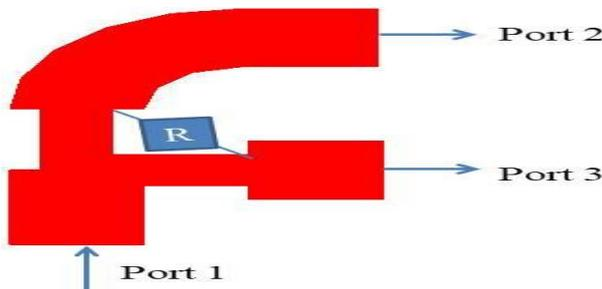
Fig. 4: Layout of the Modified 2-Way Wilkinson Power Divider
