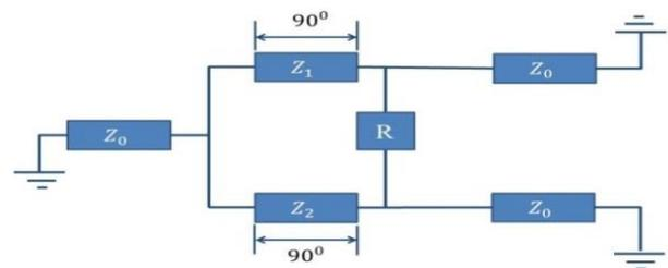
Fig. 1: Schematic Model for Wilkinson Power Divider.
