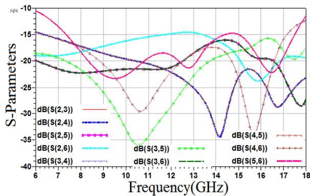
Fig. 8: Isolation of the Proposed Design
