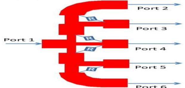
Fig. 6: Layout of the Unequal 5-Way Wilkinson Power Divider.
