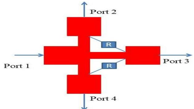
Fig. 5: Layout of the Modified 3-Way Wilkinson Power Divider
