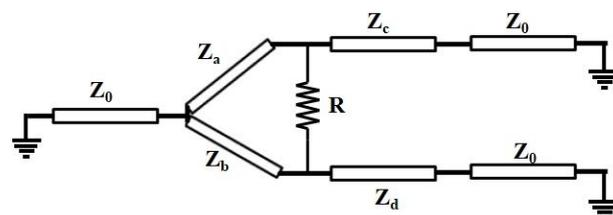
Fig. 2: Schematic Model for Unequal Wilkinson Power Divider.
